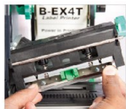
“卡扣式”打印头使装卸耗时最低
