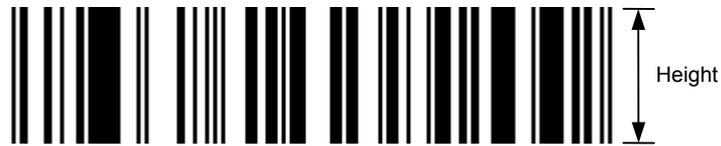
When the bar code height is 0000, bar code (including guard bars) and numerals under bars are not drawn. However, the bar code printed on the previous label is cleared.
