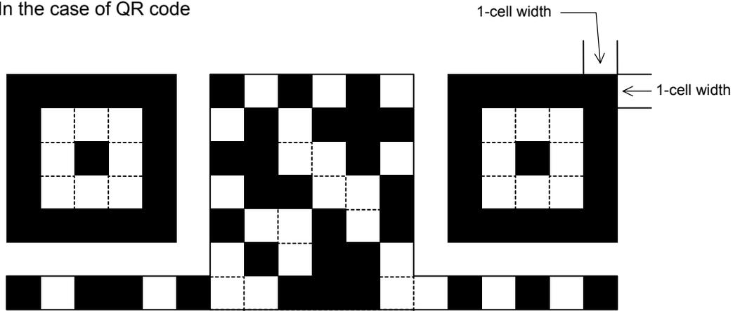
When the 1-cell width is 0, a two-dimensional code is not drawn. However, the bar code printed on the previous label is cleared.
