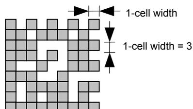
When 1-cell width is 00 for the Data Matrix or CP code, a two-dimensional code is not drawn. However, the two-dimensional code printed on the previous label is cleared.
