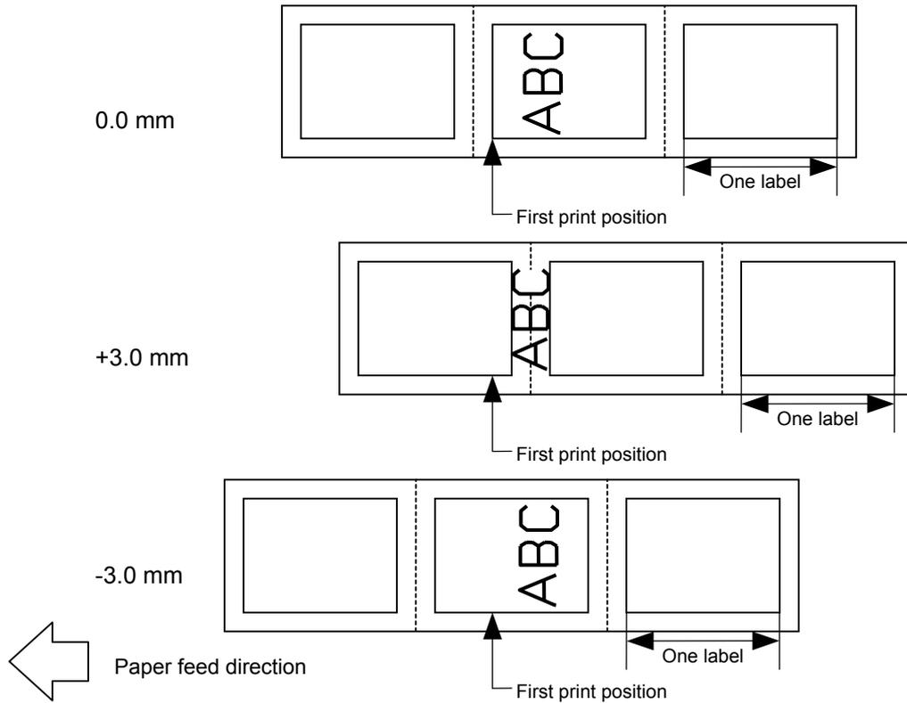
[Cut Position Fine Adjustment] (To finely adjust the cut position for shifting backward or forward)
