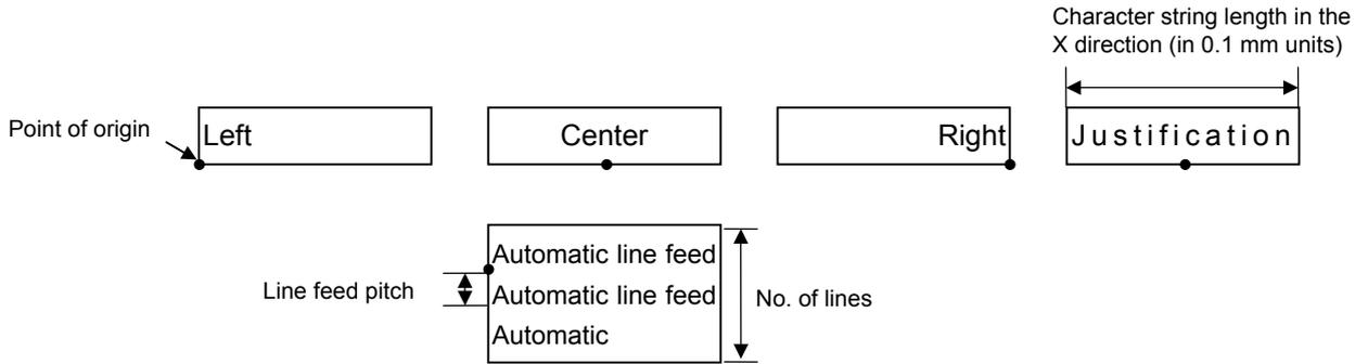
If all data characters do not fit in one line when justification and automatic line feed are designated, the following steps are performed.
