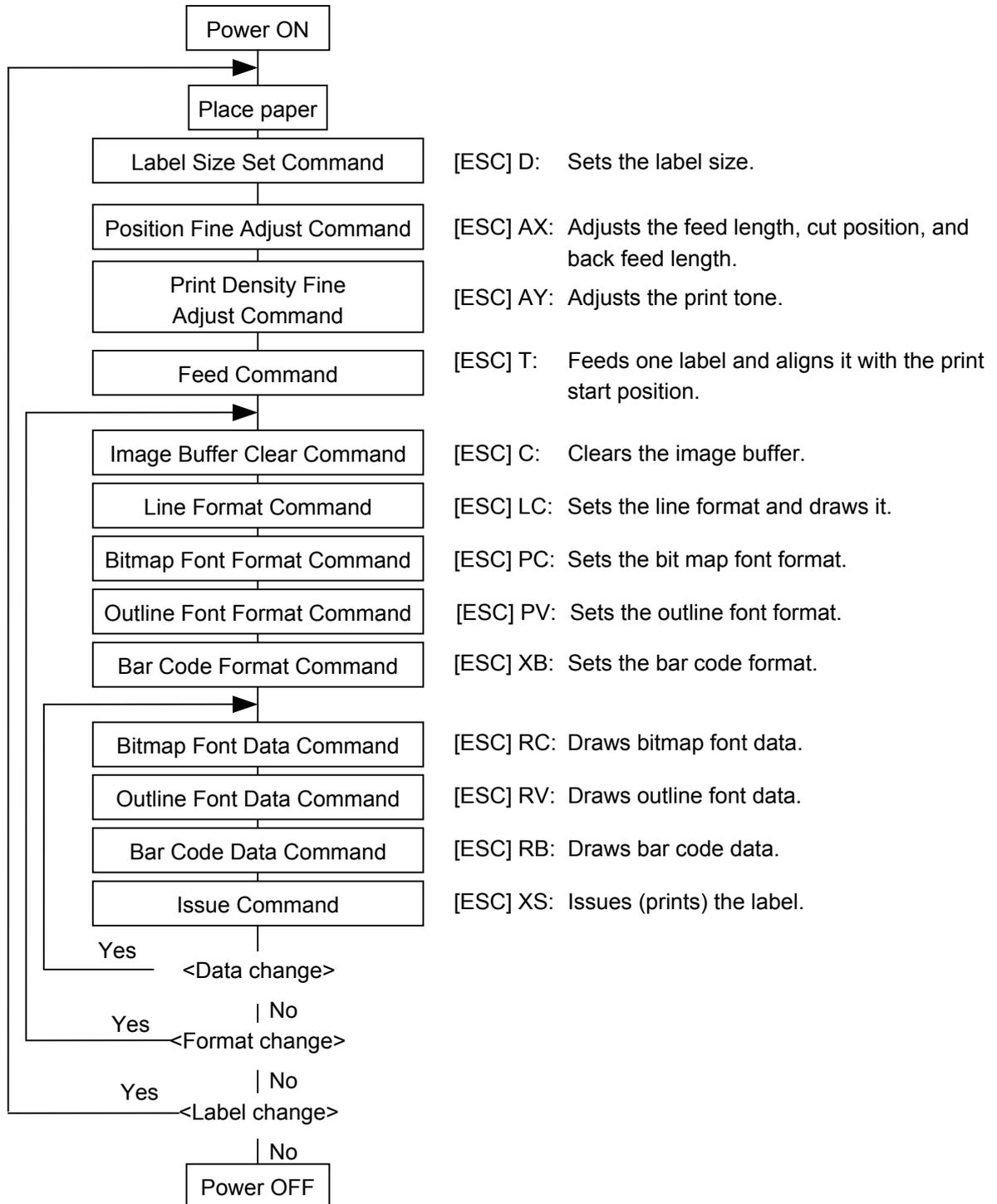
**NOTES:** (1) Whenever a paper type is changed, the Label Size Set Command and the Feed Command must be sent. When the same paper continues to be used after the power is turned off and on, the Label Size Set Command and the Feed Command may be omitted.
