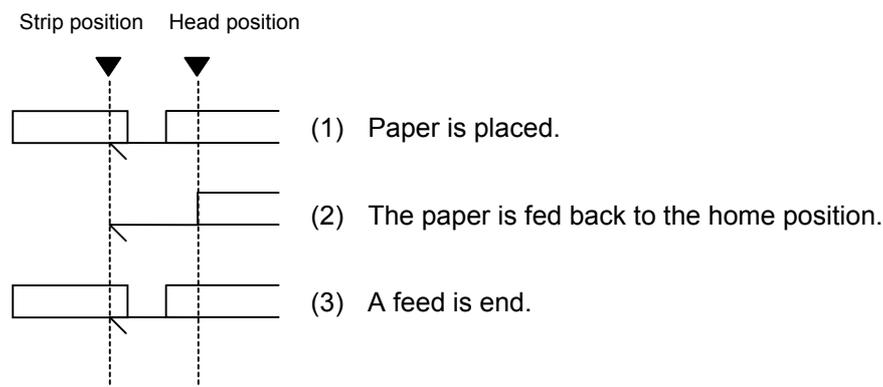
\*1 Feed mode E is different from feed mode D in the way the subsequent labels are issued. In feed mode E, labels are issued regardless of whether or not the printed label is removed.
