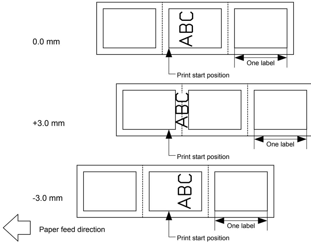
[Cut Position Fine Adjustment] (To shift the cut position backward or forward)
