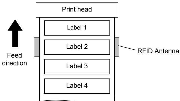
How the printer performs printing and data write when print data for several labels is transmitted to the printer is explained for each of the offset printing parameter options using the above illustration, as follows.
