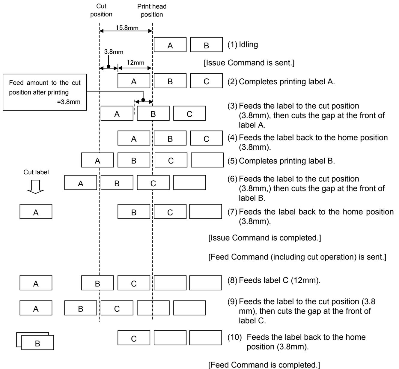
**Note:** Distance between the print head and the disc cutter: 15.8 mm
