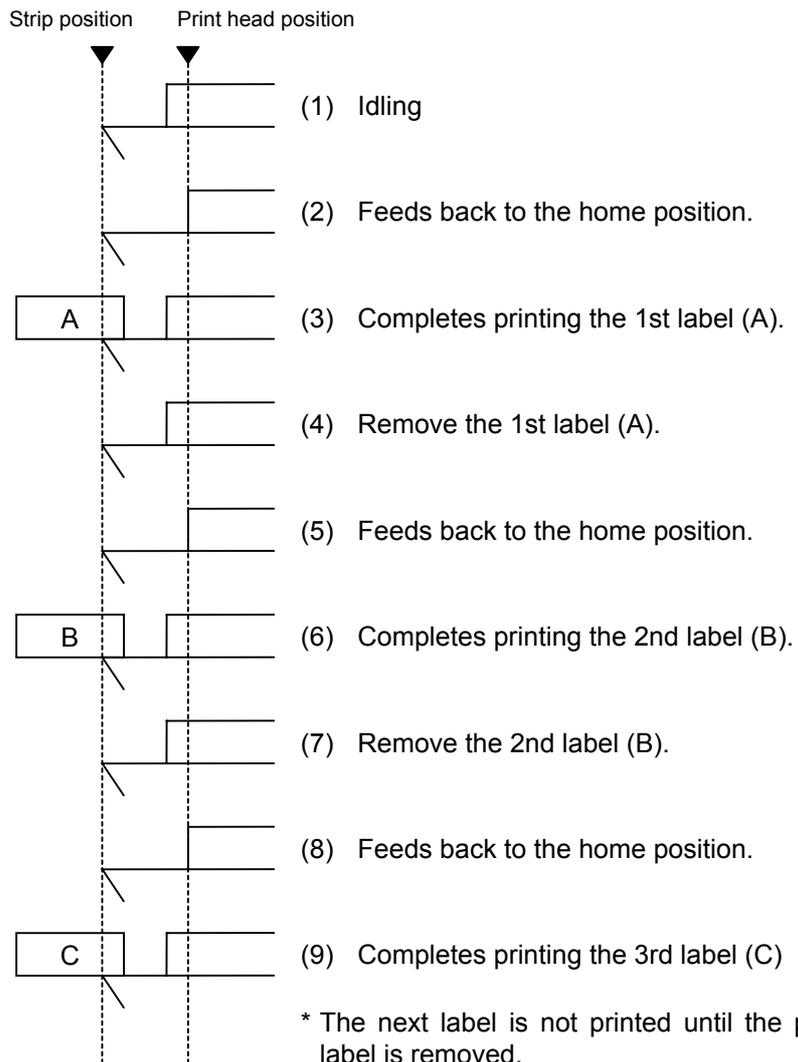
\* The next label is not printed until the printed label is removed.
