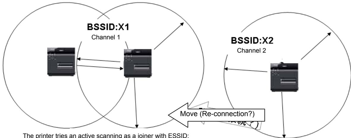
The printer tries an active scanning as a joiner with ESSID: ABC. When the printer receives a valid response from the creator, it connects to the IBSS created by the creator.
