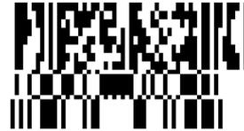
GS1 DataBar Stacked Omnidirectional
