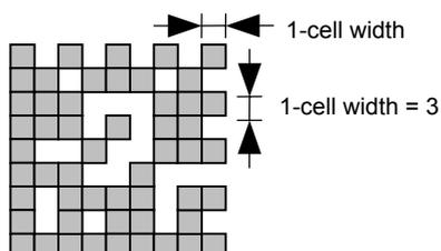
When 1-cell width is set to "00" for the Data Matrix or CP code, a two-dimensional code is not drawn. However, the two-dimensional code for the previous label is cleared.
