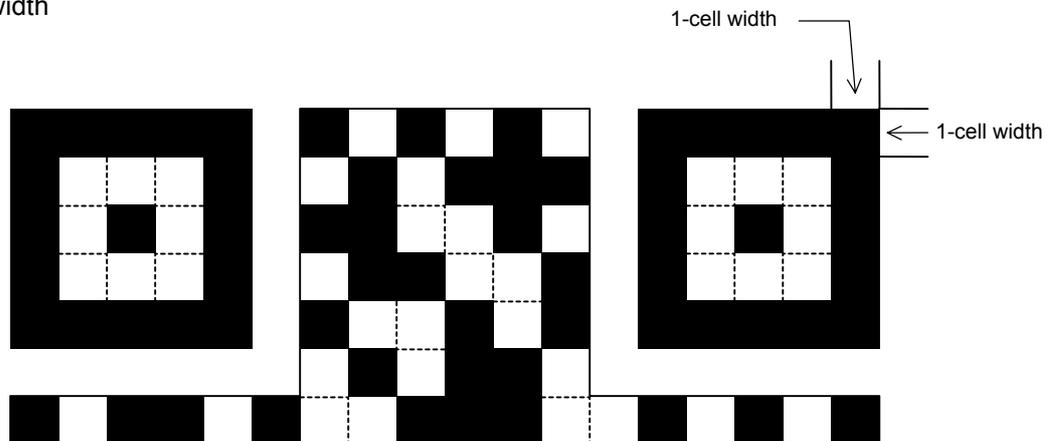
When the 1-cell width is 0, a two-dimensional code is not drawn. However, the two-dimensional code printed on the previous label is cleared.
