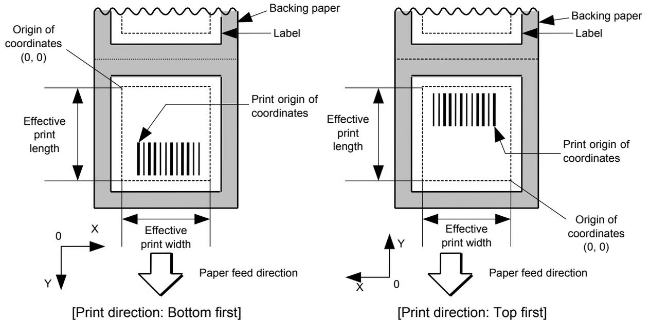
The print origin of coordinates must be set so that the bar code is drawn within the effective print area set by the Label Size Set Command ([ESC] D).
