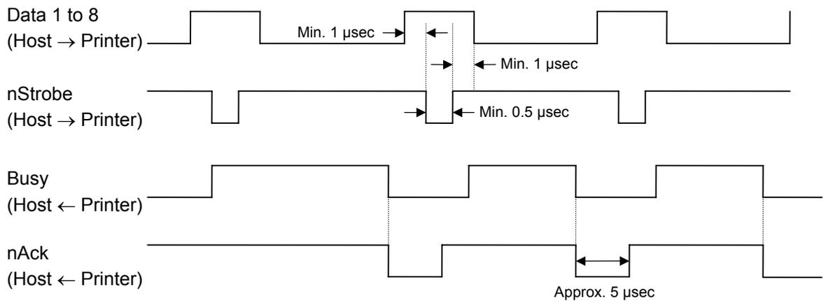
② Receiving data in the Compatibility mode when the free space in the receive buffer is 512 bytes or less:
