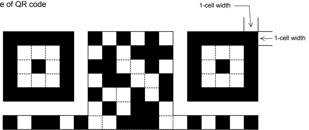
When the 1-cell width is set to "0", a two-dimensional code is not drawn. However, the bar code for the previous label is cleared.
