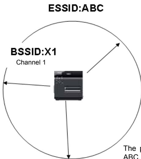
**ESSID (Extended Service Set ID):** One of the identifiers, identifying a name of a wireless access point. It is named by a user.
