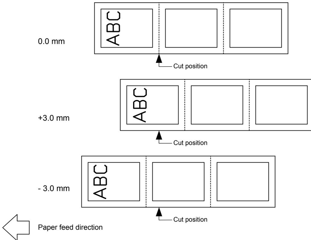
[Strip Position Fine Adjustment] (To shift the strip position backward or forward)
