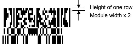
[GS1 DataBar Stacked Omnidirectional]
