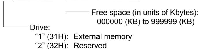
When an external memory is not inserted, "00H, 00H, 00H, 00H, 00H, 00H" is returned as the free space. When the free space size exceeds the max. value of 999999 (K bytes), it will be automatically corrected to 999999 (K bytes).
